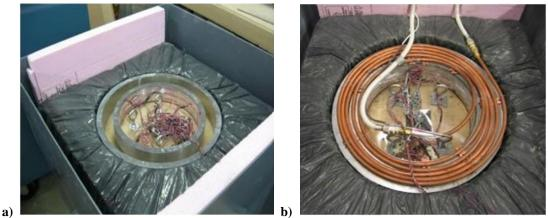
Figure 1. Dual-Ring Shrinkage a) insulation box with rings ready for mortar to be cast, and b) heating/cooling coil unit on top of cast mortar sample.
